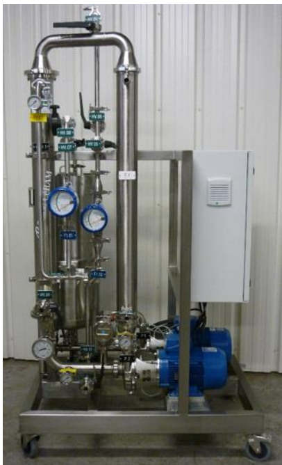
SIVA's pilot unit for seven ceramic membranes used during the tests
