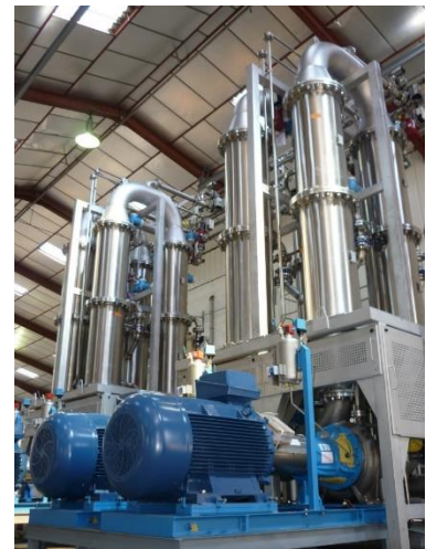
Glucose syrup clarification unit with TAMI Industries' ceramic membranes at SIVA
