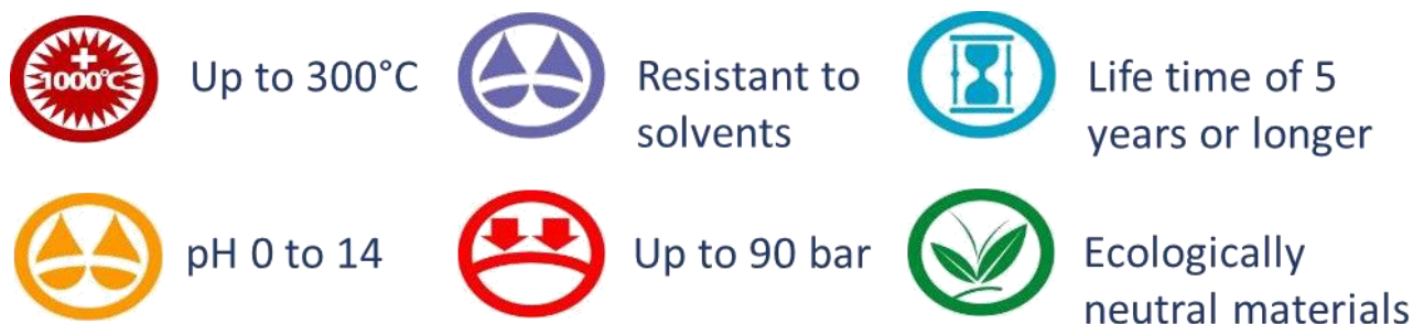
Figure 4: Summary of the key properties of ceramic membranes
